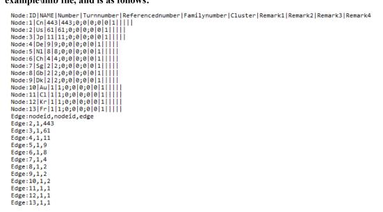
imb format data can define nodes and connections for simple visual display.
